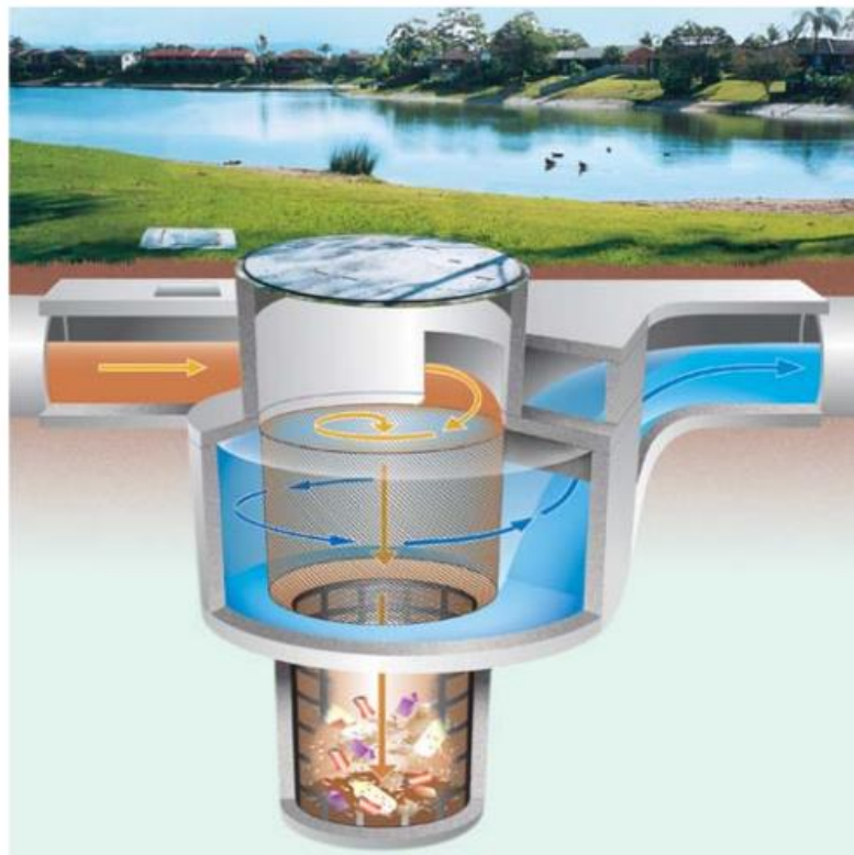
Figure 3-3 Rocla CDS Unit (source: Rocla Technical Manual)
